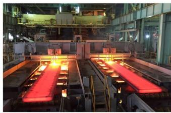
Continuous caster 4 in operation at Zhanjiang Steel's Phase I, producing zero-defect slabs in a highly efficient and low cost way
