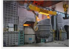
A BOF self-adaptive constraint system, with a 4-point linkage suspension system, including an oxygen lance
