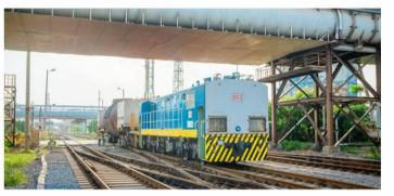
CISDI's autonomous locomotive, loaded with hot metal, traverses the railway crossing from ironmaking plant to steelmaking plant at Baowu Group's Zhanjiang Steel
