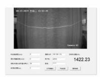
A CISDI Sigma screen shot, showing the use of machine vision to identify the belt conveyor's material flow and volume
