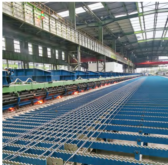
The bars being cooled on a cooling bed for the dual high-speed bar rolling line at Chongqing Steel
