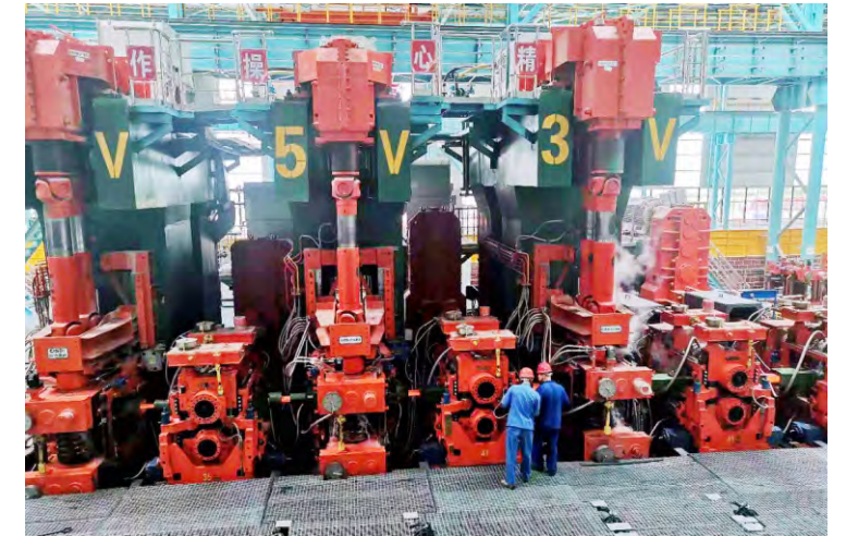
CISDI-supplied NHCD short-stress path rolling mills are hot commissioned for a high-speed wire-rod rolling line at Shiheng Special Steel in China's Shandong Province
